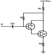
Q3. For the amplifier shown in Fig.3 using a transistor whose parameters are  $h_{ie}=1100, h_{re}=2.5\times10^{-4}, h_{fe}=50, h_{oe}=24\mu\text{A/V.Find A_I},$  A<sub>V</sub>, A<sub>VS</sub> and R<sub>i</sub>.
